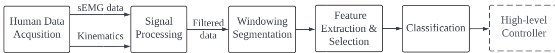
Fig. 1. Overview of the proposed research framework. The last segment of the flowchart (high-level controller) is marked with dashed lines because it is not included in this paper, however, is included in the flowchart to show how the proposed methods could be used for the control of a wearable or prosthetic device.
