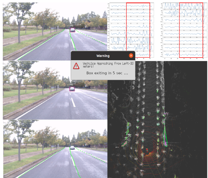
Fig. 5. A complete depiction of signals and computation results after processing. The left side shows the image data captured by the rearview camera, lane detection and object detection applied to the image. The right side shows the point cloud data at bottom and EMG data on top. The left side top image shows the fused results in one image that includes lane and object detection and the distance measured by the lidar. The red triangle in the EMG data shows the intention prediction in the continuous stream of EMG signals.
