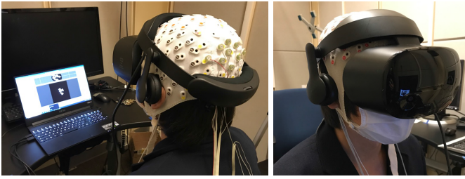
Fig. 2. Experimental environment. Participants fixed their gaze at the center of the stimulus so that it simultaneously elicits multi-focal steady-state visual evoked potentials (mfSSVEPs) and saccadic eye movements.
