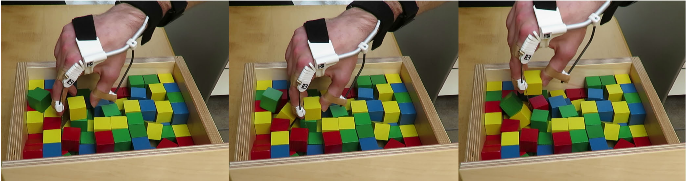
Fig. 8. Stills from the Box & Block Test of P02 showing the initial hand opening (left), actual grasping (middle) and lifting (right) of one block.
