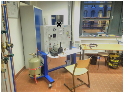
Fig. 1. Miniature steam-engine. The water is filled into the tank and heated using a Bunsen burner. The ascending steam then flows through the copper steam tubes through the one-cylinder steam machine, finally reaching the condensation tube where the steam condenses and is transported out of the system. For the active condition, the gas supply can be manipulated to manage the resulting heat using a valve. Also, the steam that runs through the steam engine can be controlled via a steam valve. All pressure and temperature values can be accessed using a dial and an LED display (marked as X).
