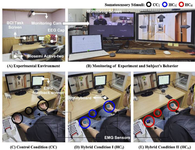
Fig. 1. Overview of experimental environment. (A) Experimental environment. (B) Control room: monitoring of experimental procedure and subject's behavior, and measuring EEG signals. (C) Control condition (CC): kinesthetic imagery without somatosensory stimuli. (D) Hybrid condition I (HC I ): somatosensory stimuli of same type (hard and rough ball). (E) Hybrid condition II (HC II ): somatosensory stimuli of different type (soft and smooth ball: left hand; hard and rough ball: right hand; soft and rough half-ball: right foot).
