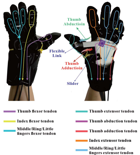
Fig. 2. Tendon actuation schematic of the hand exoskeleton. (a) Palmar and (b) dorsal views.
