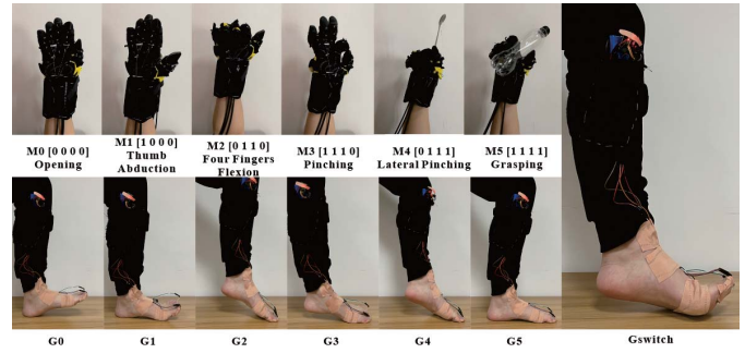
Fig. 6. Hand gestures of the hand exoskeleton corresponding to the foot gestures. The activated DOFs of the hand gestures are encoded as marked in the images below.
