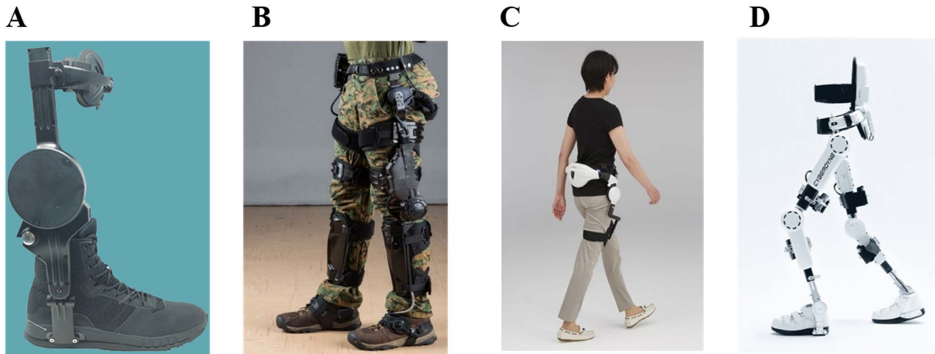
Fig. 1. The Dephy ExoBoot ankle exoskeleton (A), the Lockheed Martin ONYX knee exoskeleton (B), and the Honda Walking Assist hip exoskeleton (C) are three examples of single joint exoskeletons that augment human performance. The Cyberdyne HAL exoskeleton (D) is a three joint rehabilitation exoskeleton.
