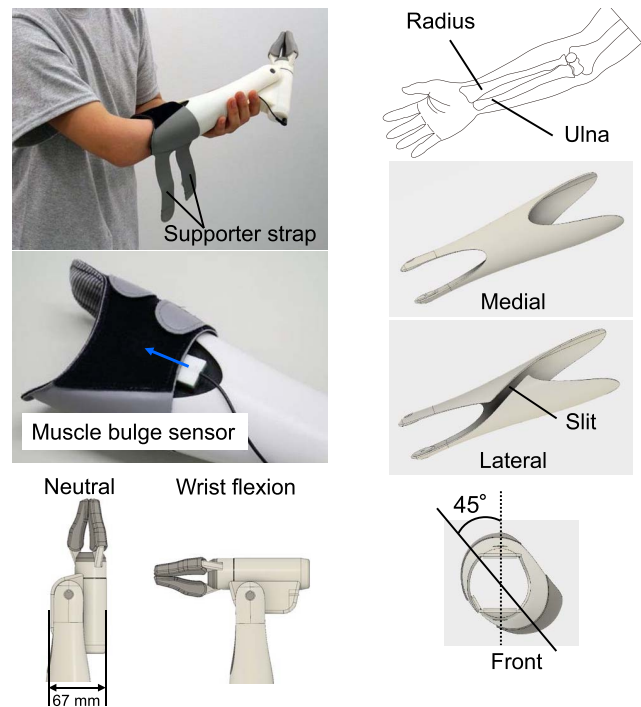
Fig. 6. Supporter socket consists of the resin socket frame and the fabric supporter. A user can wear the Finch by tightening the supporter straps.
