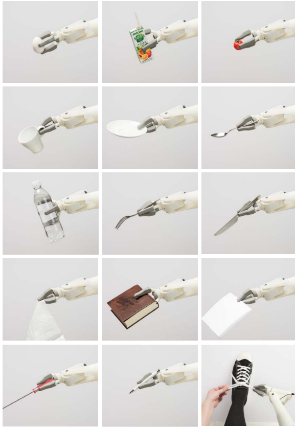
Fig. 14. Examples of daily objects grasped by the Finch. When it holds stick-like objects such as a pen, the objects are supported by three fingers and a silicone body cap.
