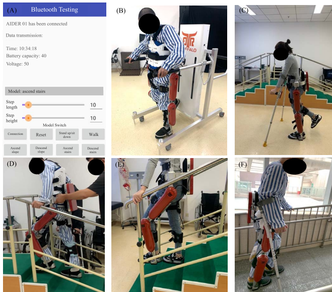
Fig. 1. AIDER powered exoskeleton illustration used in this study. (A) a mobile phone application; (B) walk with body-weight-supported AIDER system; (C) walk in exoskeleton; (D) go upstairs in exoskeleton; (E) go downstairs in exoskeleton; (F) ascend slope in the exoskeleton.
