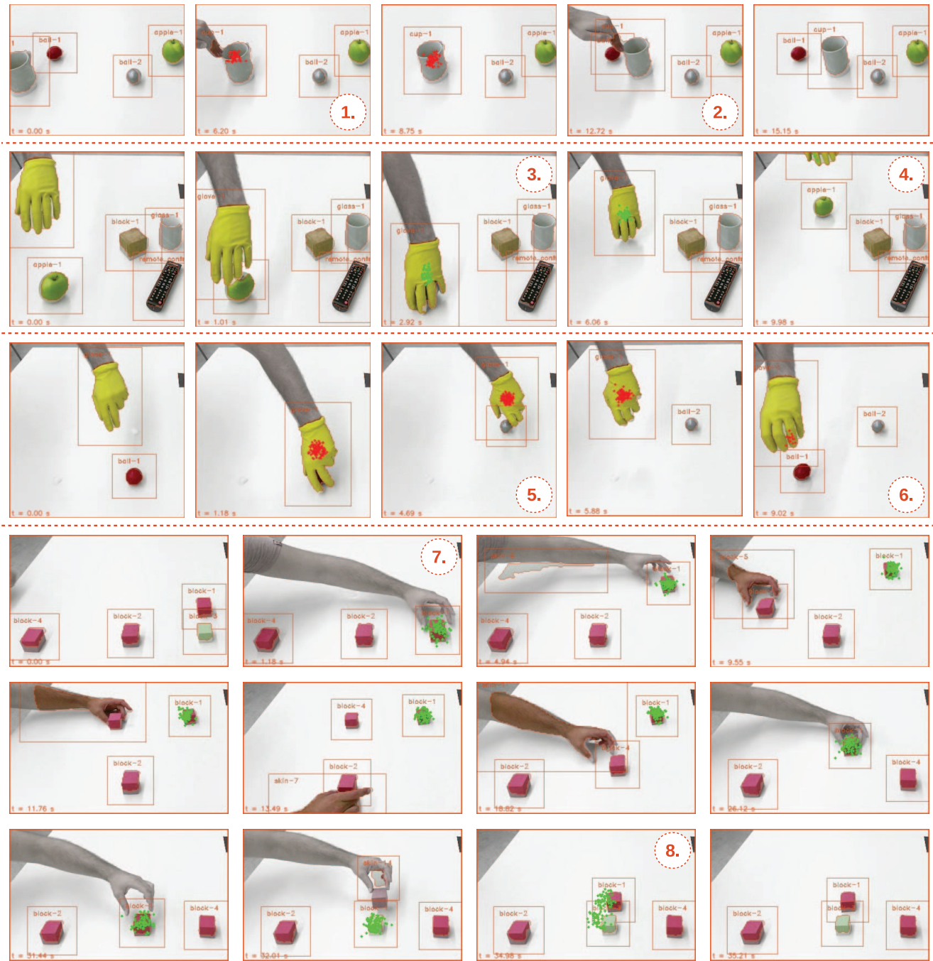
Fig. 6. Examples of screen-shots captured during the execution of stated scenarios. Visual perceived anchored objects are symbolized with the unique anchor id (e.g., ball-2), while occluded hidden objects are depicted by plotted particles that represent possible positions of the occluded object in the inference system. Rows in order from the top: First row example of simple occlusion where a ball is hidden behind a cup, second row depicts the movement of an occluded object where a glove (or human hand) is occluding while moving an apple, third row similar example of moving an occluded object where a glove is occluding while moving a ball (ball-1), but in this case is also another ball object (ball-2) introduced during the execution of the scenario, fourth row–sixth row illustrate a shell game scenario where a smaller object (block-3) is hidden under one of three identical containers (block-2), and where the containers, subsequently, are shuffled around.
