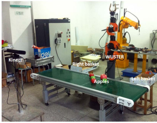
Fig. 12. Experimental platform of apple sorting robot system.
