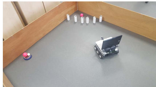
Fig. 2. Koala robot used in our experiments. Additionally, the light movable objects from experiment 2 and a moving “prey” resource from experiment 3 can be seen at the top and left of the figure, respectively.
