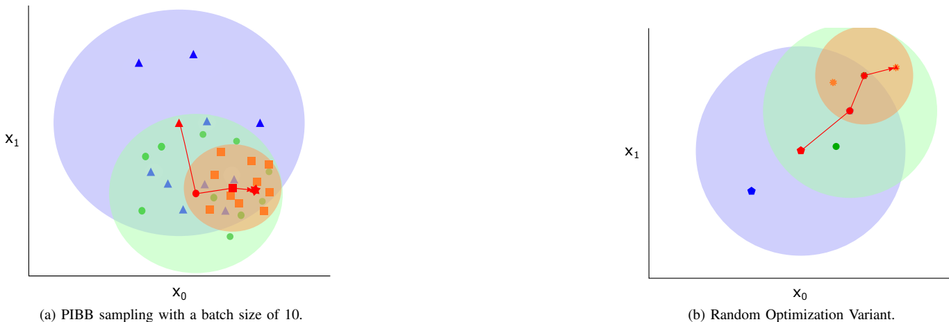
Fig. 2: Schematic visualization of PIBB sampling (left) and the Random Optimization sampling (right). Both schemes show the optimization for 3 epochs in a 2-dimensional representation space. Blue, green and orange symbols depict the samples of first, second and third epoch respectively. The samples lie in the exploration radius, marked as colored ellipses around the current mean for each epoch. Red symbols show the means of the batches. Red arrows indicate update steps.
