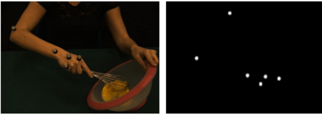
Fig. 1. Left image shows a frame of action eggs from a frontal point of view, and the right image shows its PLD. PLDs correspond to the positions of the markers.
