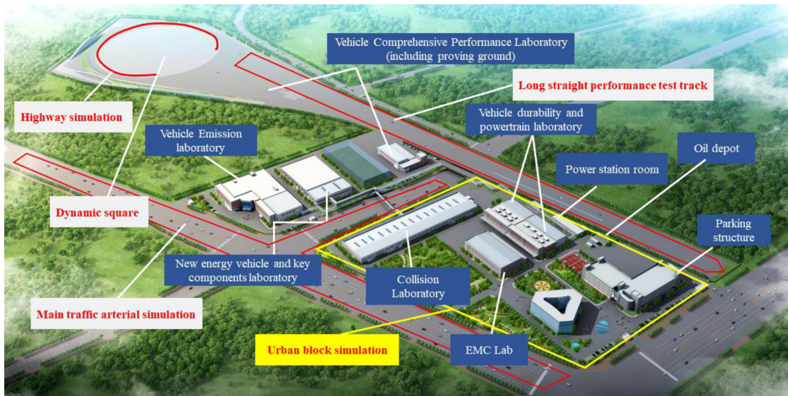
Fig. 2. The PTAVC's Proving Ground at CATARC Automotive Test Center (Guangzhou), including 195000 square meters of road area and 90000 square meters of test laboratories.
