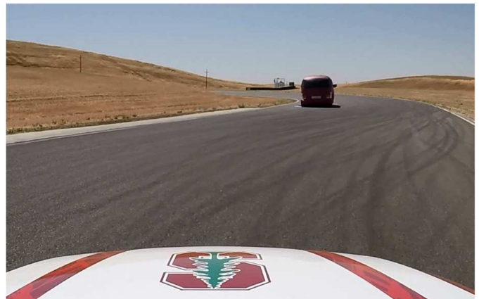
Fig. 5. Picture from test with obstacle location marked by mock vehicle.
