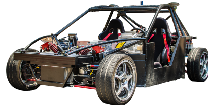
Fig. 1. X1, the drive-by-wire, student build research vehicle. The drive-by-wire capabilities are well suited to driver assistance system testing, allowing the system to override driver commands when necessary for safety.
