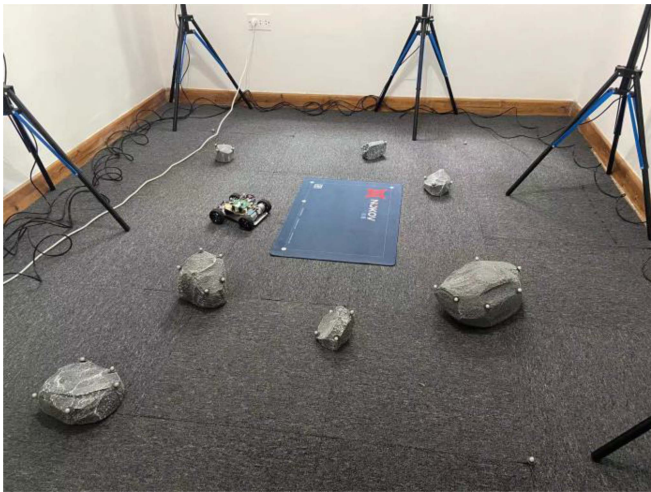
Fig. 7. An indoor workspace and a small-scale autonomous vehicle platform deployed for the field tests.
