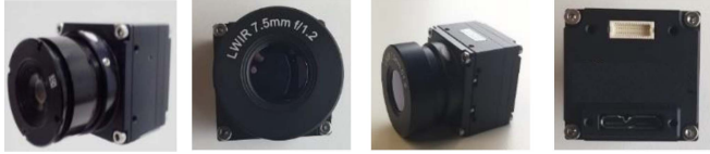
Fig. 1. LWIR thermal imaging module images from different view angles.
