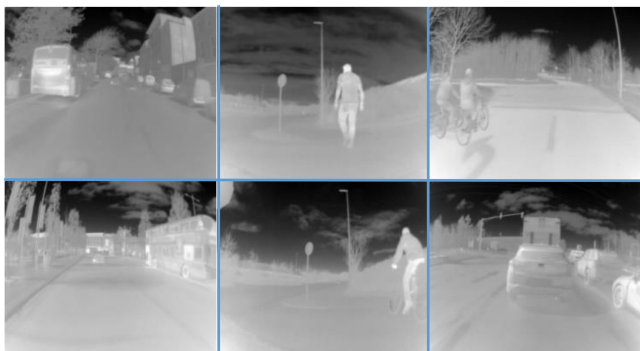
Fig. 11. Six different thermal samples acquired using LWIR 640 \times 480 prototype thermal camera showing various class objects.
