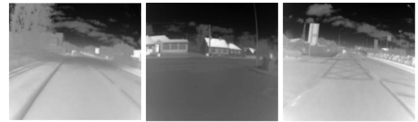
Fig. 7. High-quality thermal frames after applying the shutterless calibration algorithm and image correction methods.
