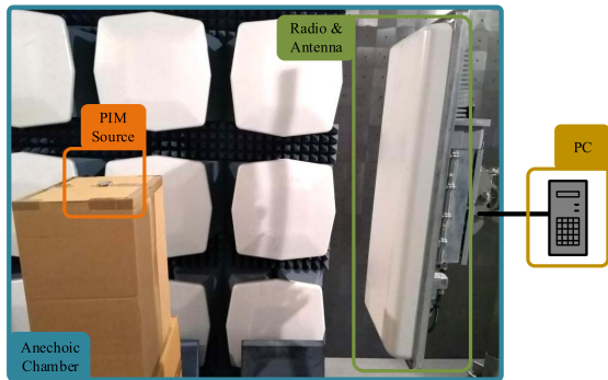
Fig. 2. Measurement setup with the relevant parts of the system highlighted.
