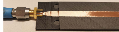
Fig. 1. Photograph of the test assembly for the proposed technique. A puzzle-like launcher (black material) is used at each end as an intermediate element between the end-inserted coaxial connector and microstrip line on the substrate-under-test (gray material). Launchers are then de-embedded to provide the measured S -parameters referenced at the test material edges.
