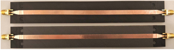
Fig. 3. Assembled test lines for FDM printed substrates: reference black PLA and magnetic iron PLA. The use of copper tape enables a seamless realization of the microstrip conductor.
