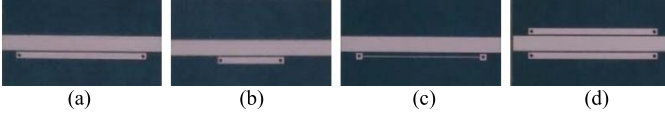
Fig. 3. Top views of four different structures for comparison. (a) Fundamental VSRR structure. (b) VSRR with the short length ( L_1 = 10 mm). (c) VSRR with the small width ( W_2 = 0.15 mm). (d) Dual VSRRs ( n = 2 ).
