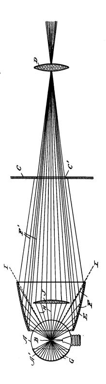
The obvious method would be to avoid the light absorption loss by using only thin lenses, and to usefully employ light now lost by reflection. Not only would thin lenses avoid absorption loss, but also the prismatic fringes at the blunt-angled edge of the lens.
