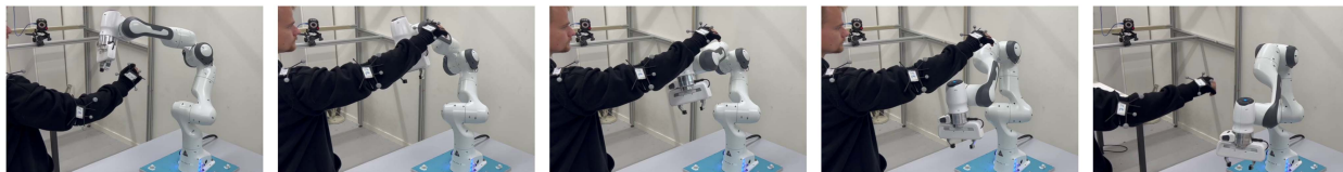
Fig. 4. Snapshots of a reaching task with the human upper body as an obstacle approximated with a collection of 30 spheres. See multimedia attachment .
