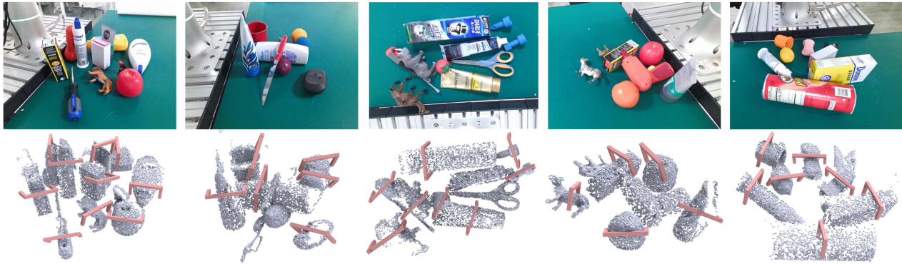
Fig. 7. Visualization of the detected grasps in cluttered scenes. Our method is able to produce high-quality grasps on objects with complex geometry and heavy occlusion, thanks to the guidance of symmetry estimation.
