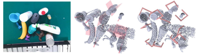
Fig. 1. SymmetryGrasp couples the detection of symmetry and grasp into a unified framework. Given a single-view RGB-D image (left), it takes advantage of the estimated symmetries (middle) to determine the feasible antipodal grasps (right), greatly increasing grasp quality and generality.
