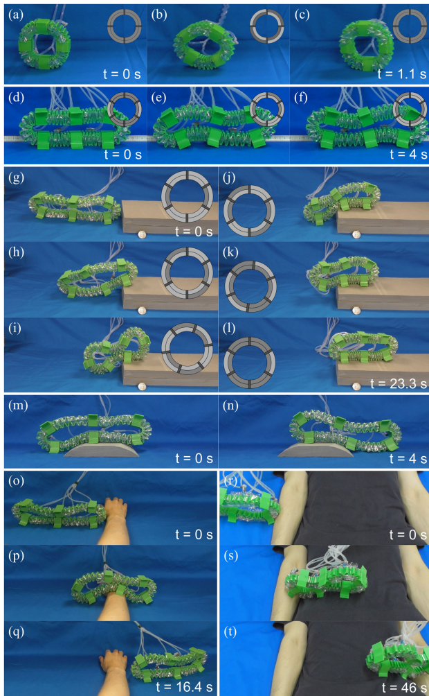
Fig. 7. Sequential Images of results for locomotion experiments. (a-l) Each image stands for one state input, and start and finish time are shown in the first and last images, respectively. Pressure input is indicated with dark gray = -60 kPa and light gray = atmosphere. (a-c) Rolling locomotion with four segments and two inputs. (d-f) Traveling wave locomotion with six segments and six inputs. (g-l) Step climbing with three inputs. (m-n) Passive compliance while overcoming small obstacles with three inputs. (o-t) Climbing the human body while keeping a soft touch.
