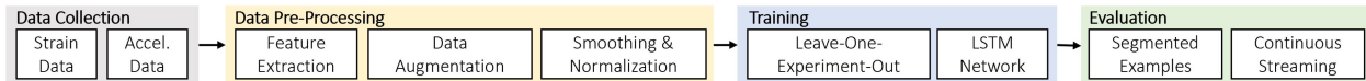
Fig. 5. The pipeline processes collected training data to create a neural network that can classify segmented examples or streaming real-time data.
