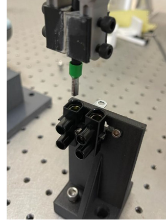
Fig. 10. Experimental system to evaluate generalization to semi-flexible pegs: inserting a 4[mm] electrical wire with crimped terminal into a connector with non-circular cross section 5–6[mm] diameter and \pm 2.5 [mm] errors.
