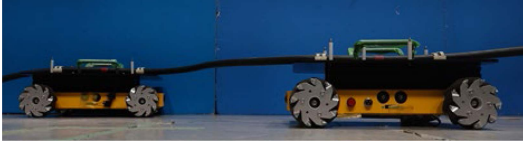
Fig. 4. Deflection of a cable between two vehicles.
