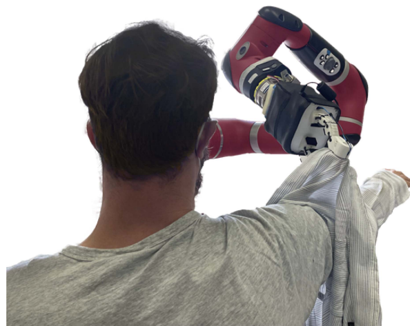
Fig. 1. The dressing setup, composed of a collaborative robot and the DressGripper, assisting a person in wearing a shirt.
