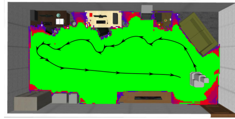
Fig. 6. Example of disinfection in a simulated environment. Green cells are the ones in the reachable space that already received more than 100% of the desired UV-C dose in the initial passage through the environment.
