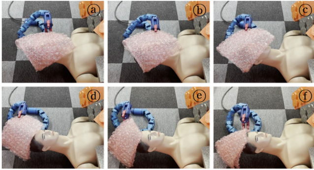
Fig. 13. Snake robot rescue operation experiments with gripper module.
