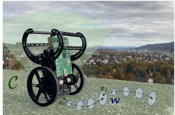
Fig. 1. Safety-critical systems require fast and tractable control algorithms. These should stabilize the system, while always remaining safe. For instance, the mini-Segway shown in the figure must follow a reference position without falling down, i.e., satisfy safety bounds on the pitch angle at all times.
