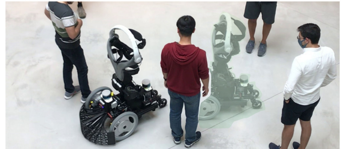
Fig. 1. The robot Qolo is passing between pedestrians using the proposed reactive controller (from right to left).
