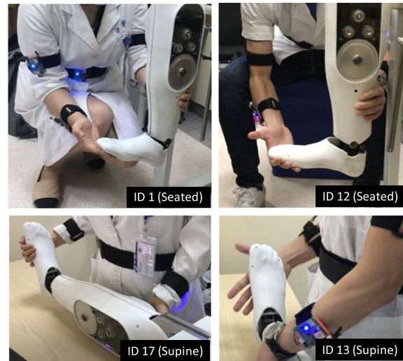
Fig. 4. Four subjects interacting with the simulator in two testing configurations that represented a patient in a seated or supine position.
