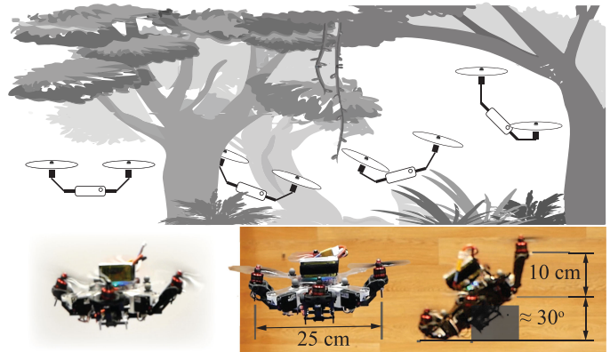
Fig. 1. The TiltDrone prototype in tilted horizontal, level, and tilted hovering flight (bottom left to right). The morphing TiltDrone can tilt up to 30 degrees, allowing it to traverse narrow areas such as dense foliage in forest environments (top).
