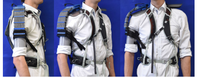
Fig. 9. Wearable proof-of-concept prototype worn by a healthy subject. This figure illustrates the actuator's potential to achieve close alignment to the body and an overall small size of the resulting assistive device.
