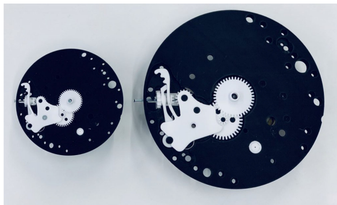
Fig. 2. Scaled-up watches 3D printed from CAD drawings: 3.5× and 5.8× bigger.
