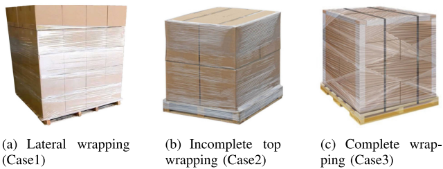
Fig. 2. Examples of different wrapping cases: the film covers only the lateral surface of the pallet (a), the film also covers the top surface partially (b), the film covers the lateral and the top surface entirely (c).
