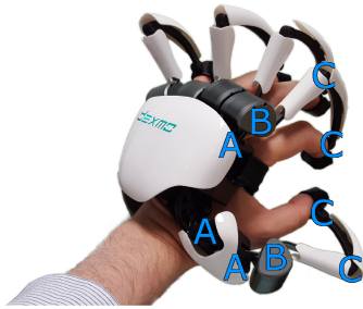
Fig. 1. The Dexmo glove, annotated with the joints that are sensed but not actuated (A), sensed and actuated (B) and not sensed or actuated (C) for the Index finger and Thumb. Other fingers have identical arrangements to the Index finger.
