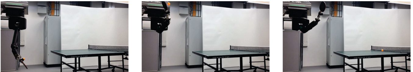
Fig. 5. A successful rollout during real robot experiments. The ball is initially on top of the egg-holder and during the movement, as a result of the acceleration of the arm, it takes-off from the robot, to be later hit by the racket towards the table. The arm then decelerates towards a safe resting posture.
