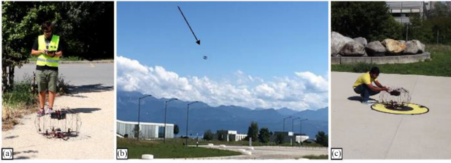
Fig. 1. Three phases of delivery on the EPFL campus. (a) The PackDrone just before take-off at the sender location. The sender is operating the software from a tablet. (b) The drone is flying above the EPFL campus. (c) The drone in a recipient location. The recipient is unloading a parcel.
