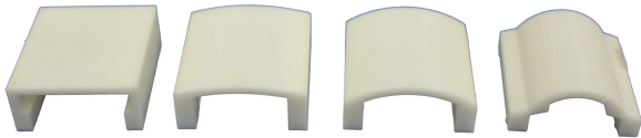
Fig. 5. Picture showing 3D printed stimuli created for this work. Each has a different radius of curvature to test ability to cope with objects of different shapes. The apex height of each object is the same (20 mm).
