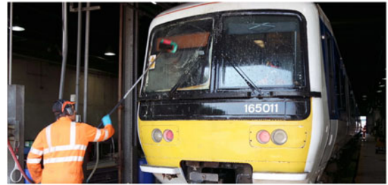
Fig. 1. Depot operative manually cleaning the front panels of a diesel train. Wembley depot, London. 9th June 2016.
