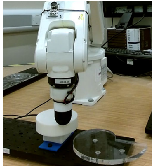
Fig. 1. Tactile robotic system, comprising a tactile fingertip (the TacTip) mounted as end effector on a 6-DOF robot arm.
