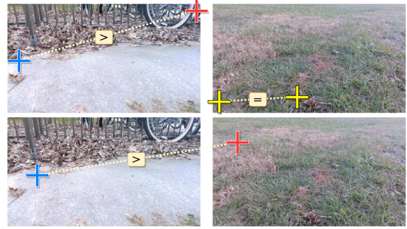
Fig. 2. Illustration of our annotation strategy on the WayFAST dataset [4], showing intra-image labeling (top) and cross-image labeling (bottom). Yellow crosshairs indicate both points in a pair are equally traversable, while the blue point is more traversable in pairs with blue and red crosshairs.
