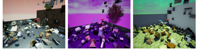
Fig. 3. Examples of the training environment randomization. The tracker (blue) and the target (red) MAVs are spawned in a large room with randomized characteristics.
