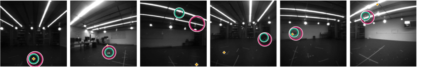
Fig. 4. LED-P-30 with \lambda = 0.001 (small green circle), BAS-30 (yellow cross) predictions and ground truth (large magenta circle) on frames taken from \mathcal{Q} with the drone's LEDs turned on (first three) and off (last three), and featuring different camera exposure settings.
