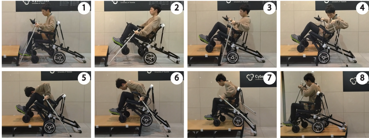
Fig. 8. Sequence of 23 cm step climbing: 1. Placing the canes in front of the step. 2. Lifting the front wheels by pushing the canes. 3. Driving forward the wheelchair. 4. Placing the canes behind the wheelchair. 5–7. Lifting the rear wheels by pushing the canes. 8. Driving forward the wheelchair to engage the passive add-on mechanism on the step.
